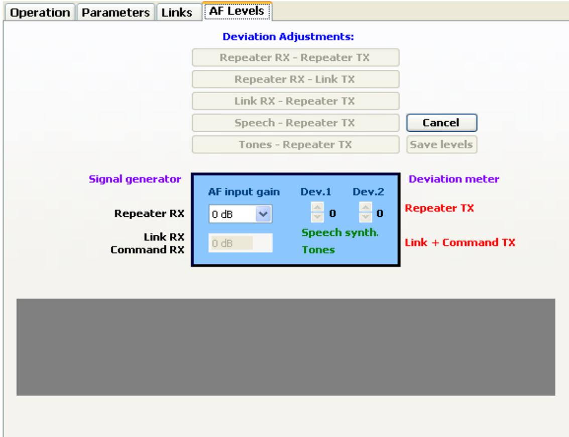
The AF signal path through the controller is linear, no de/pre-emphasis.
