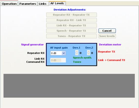
The AF signal path threw the controller is linear, no de/pre-emphasis.
